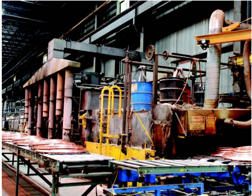
The annealing furnace allows for the heat treatment of metal to obtain softness and ductility.
